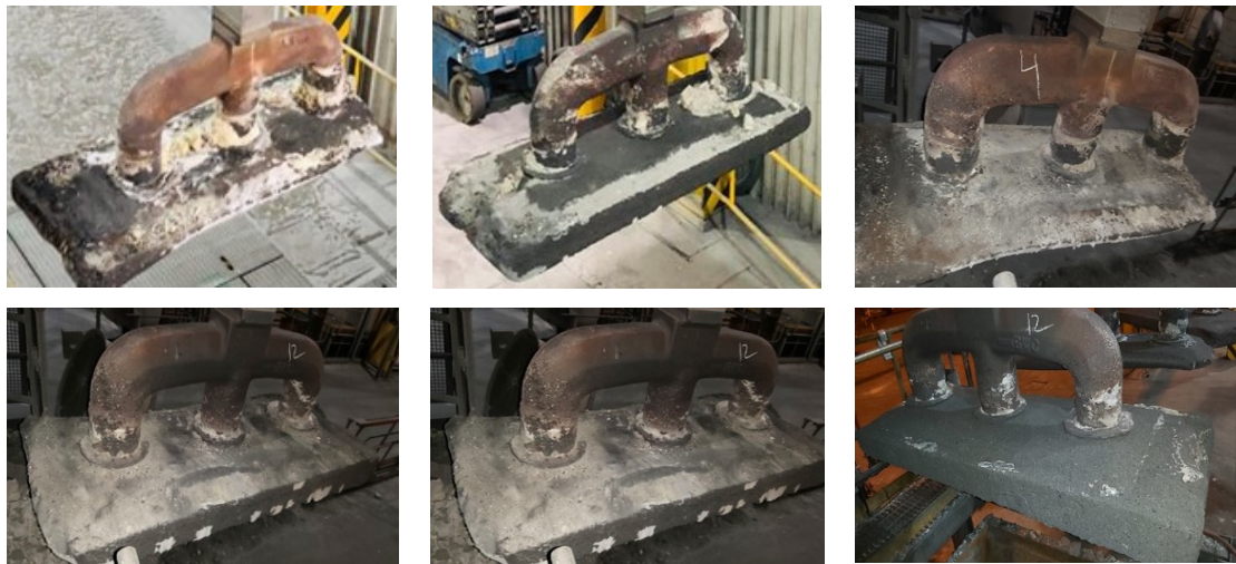
Figure 2. Images of butts with bath presence after cleaning.
